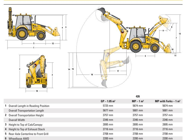
Dimensions and performance Dimensions and performance specifications shown are for machines equipped with 12.5/80-18 front tires, 16.9-28 rear tires, standard cab, standard stick with 610 mm standard duty bucket, and standard equipment unless otherwise specified.
